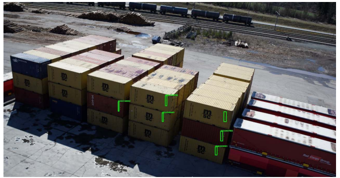
Fig. 2: Aerial view of a container stack as seen by a drone with detected container IDs in green
